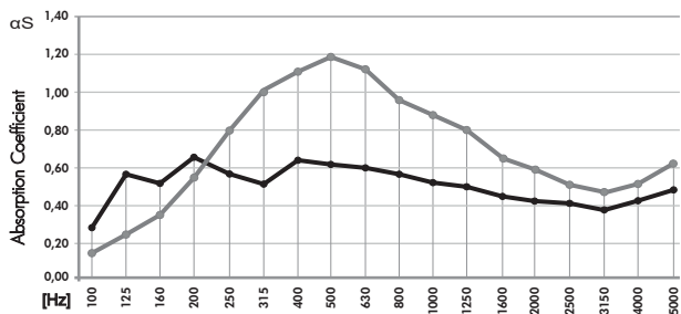
ABSORPTION COEFFICIENT: Values in accordance with the standards, EN 20654, ASTM C423 and EN 11654.
