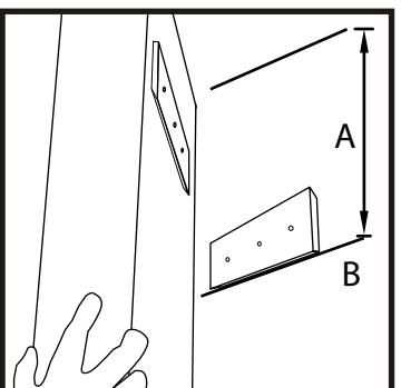
Then fit the panel into the mounting accessory.
