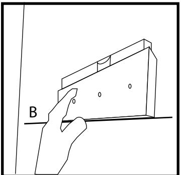
Center the accessory on the wall inserting a pencil through the wooden accessory's holes to mark the needed points on the wall.
