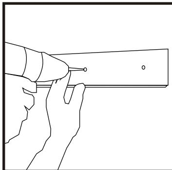
Drill the holes on the wall. Insert the nylon plugs in wall and attach the accessory with a screwdriver
