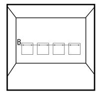
With a level define the "B" line, then mark on it the measured spacing, and two suspension points per panel on the wall. After verifying all measure-
