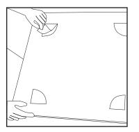
Then apply as shown in grey, the definitive PU mounting glue without solvents, for permanent applications (not-included). Apply the cords of glue marked in grey as shown on this left example image.
