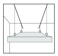
Depending on the size of the panel 2 or 3 persons can be required to suspend it. Always ensure clean and gently handling as panel finishings can be fragile. Secure the wires to the hooks on the panel to suspend it.
