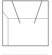
1st method: From the horizontal suspension wires install vertical wires, or
