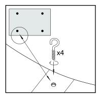
Accessories' kit; the product is supplied with the necessary accessories. Optionally suspension wires on the right are sold separately and can be made available upon demand. On the back of the panel, locate and measure included (cavities) mounting accessories distances.
