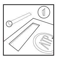
Glue and removable wooden mounting stripes are not includsold separately demand. Ensure to use mounting glue without solvents. Check the right position and try to place the removable mounting stripe to check that everything is ok to proceed. With mounting glue, cover enough area to glue the removable mounting stripe on the back of the panel, on the specific area for that (rectangular void). Confirm the positioning before the glue dries.
