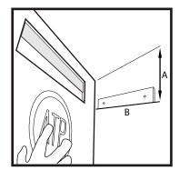
On the wall, you can use mounting glue to place the other removable mounting stripe or it can be installed with sleeves and screws.
