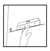
Center the accessory on the wall inserting a pencil through the wooden accessory's holes to mark the needed points on the
