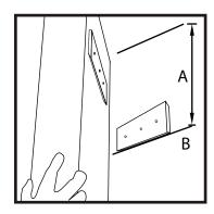
Then fit the panel into the mounting accessory.
