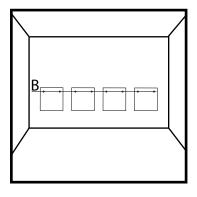
With a level define the "B" line, then mark on it the measured spacing, and two suspension points per panel on the wall.
