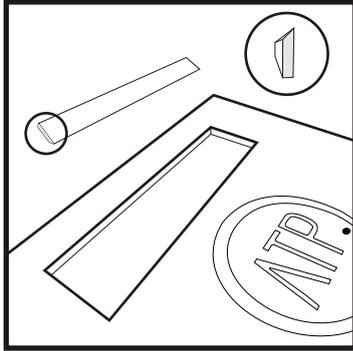
Glue and removable wooden mounting stripes are not included, sold separately upon demand. Ensure to use mounting glue without solvents. Check the right position and try to place the removable mounting stripe to check that everything is ok to proceed. With mounting glue, cover enough area to glue the removable mounting stripe on the back of the panel, on the specific area for that (rectangular void). Confirm the positioning before the glue dries.
