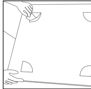
Then apply as shown in grey, the definitive PU mounting glue without solvents, for permanent applications (not-included). Apply the cords of glue marked in grey as shown on this left example image.
