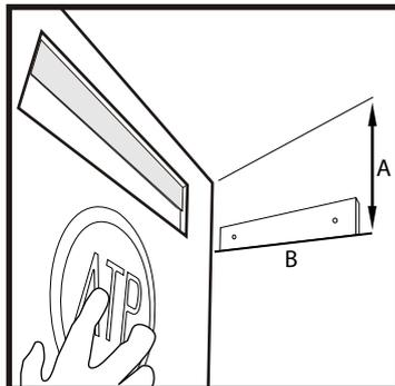
On the wall, you can use mounting glue to place the other removable mounting stripe or it can be installed with sleeves and screws. Then fit the panel into the mounting accessory and it's done!
