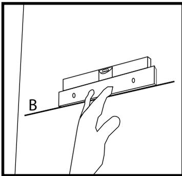
Center the accessory on the wall inserting a pencil through the wooden accessory's holes to mark the needed points on the wall. Drill the needed holes on the wall. Insert the nylon plugs in wall and attach the accessory with a screwdriver.
