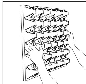
Place the panel on the surface and press it gently and homogeneously during the mounting glue's curing time, average aprox. time 2 hours.
