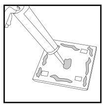
NOTICE: Adhesive time is entirely dependant on the weight of the panel to be glued. Always consult the mounting glue specifications. Adhesive gluing times can vary with humidity and temperature. Make sure that the room temperature and humidity is within the acceptable product values available on our website.
