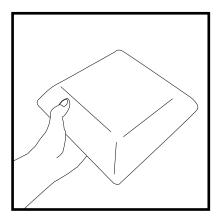
Prior to application, always clean all surfaces before applying any glue, ensuring them free of dust or grease. A vacuum cleaner can be used to clean any dust before any glue.
