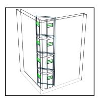
Use a level bubble tool to level the supporting "L" accessories onto the wall to ensure they are horizontally leveled and attach them as shown.
