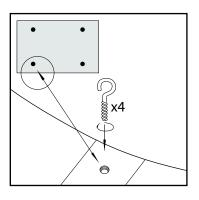
Accessories' kit; the product is supplied with the necessary accessories. Optionally suspension wires on the right are sold separately and can be made available upon demand. On the back of the panel, locate and included (cavities) measure mounting accessories distances.
