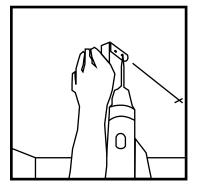
Use a screwdriver to attach the 4 mounting L-shaped metalic accessories to the ceiling. Fit the panel between the L-shaped metalic accessories and screw them to the sides of the panel.
