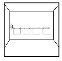
With a level define the "B" line, then mark on it the measured spacing, and two suspension points per panel on the wall. After verifying all measure-
