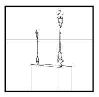
Measure the ceiling and mark points as needed to install suspension metal hooks; or horizontal suspension cables on the ceiling
