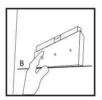
Center the accessory on the wall inserting a pencil through the wooden accessory's holes to mark the needed points on the wall.
