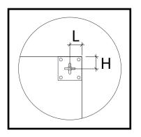
Measure"L" and "H" distance on the back of the panels on both sides.
