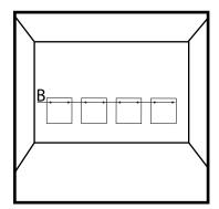
With a level define the "B" line, then mark on it the measured spacing, and two suspension points per panel on the wall. After verifying all measurements, drill 2 holes on the wall per panel, install both sleeves and 2 screws. Leave the tip of the screws aprox. 5 mm from the wall.
