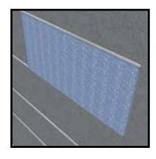
Fit each panel onto the mounting bars by carefully applying some pressure to the panel as needed, while protecting front surface finishings. Do the same for the remaining panels as shown.
