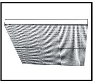
**NOTICE:** If and when necessary, panels can be cut with standard wood cutting tools. For uneven wall dimensions, smaller panel areas are normally installed near the corners for aesthetic reasons. Adhesive time is entirely dependant on the weight of the panel to be glued. Always consult mounting glue specifications. Adhesive gluing times can vary with humidity and temperature. Make sure that the room's temperature and humidity are within the acceptable product values available on our website.
